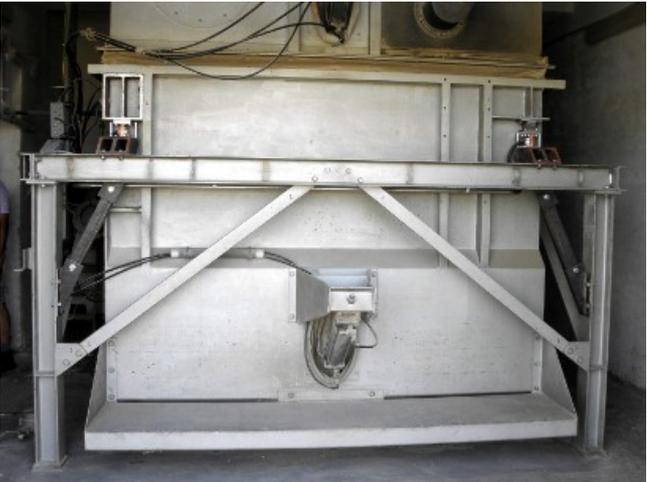
Weighing bin after conversion (on weighing modules)
