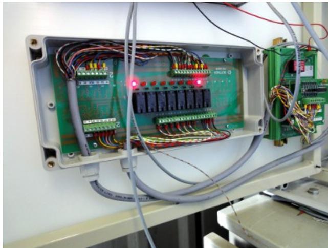
Relay box for outputs and feedback control
