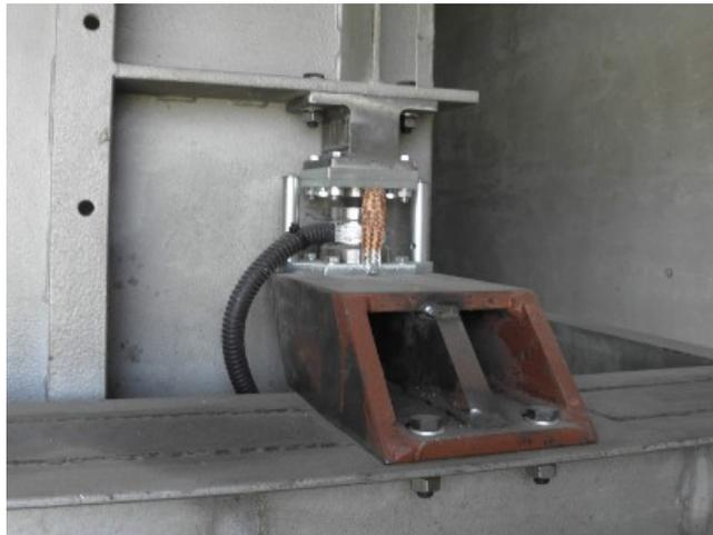
Weighing module, model B-DJ-M5, with adapter
